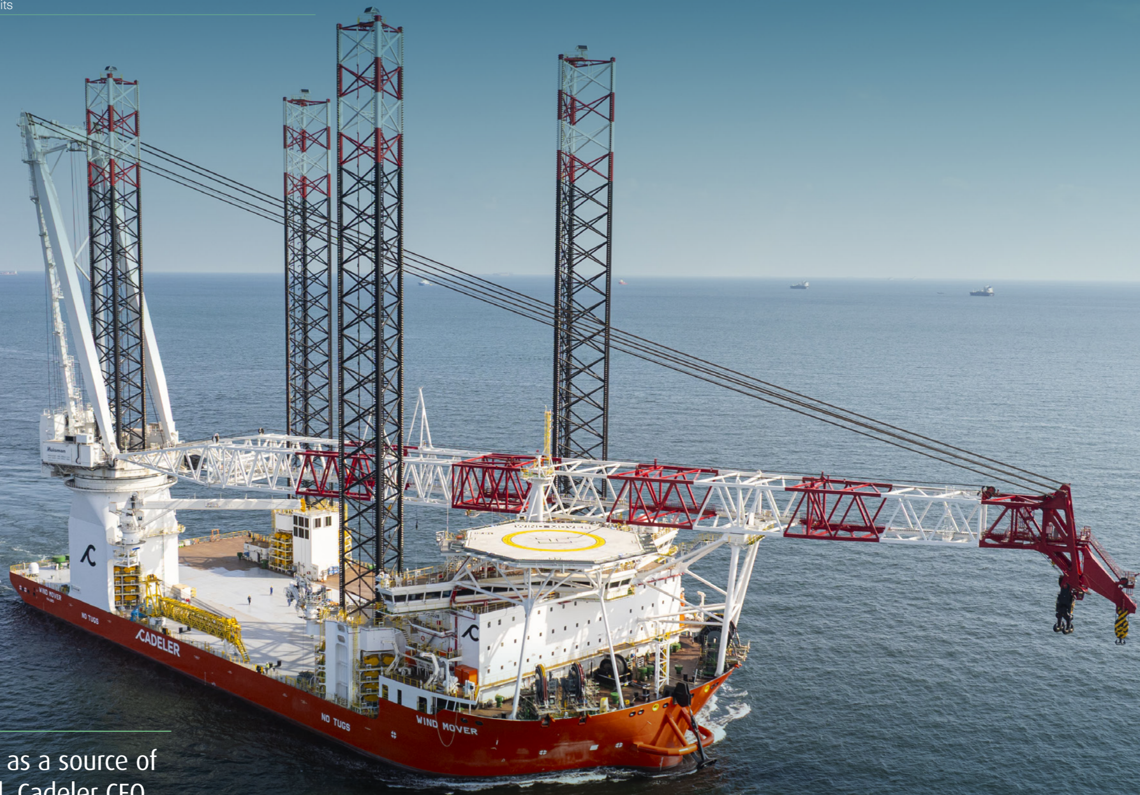
Wind Mover, Cadeler's second M-class vessel, purpose-built to install the next generation of offshore wind farm components, and currently installing 15MW Vestas turbines at the Baltic Power offshore wind farm in the Polish Baltic Sea.
